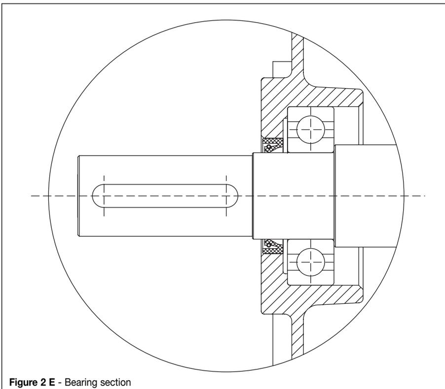
Figure 2 E - Bearing section
