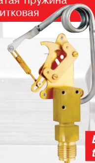
Elastic element, Bourdon tube type, C-form
